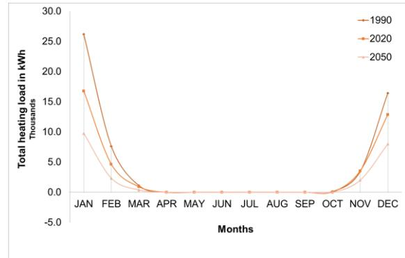
Figure 2: Heating load in kWh for DA HQ building
