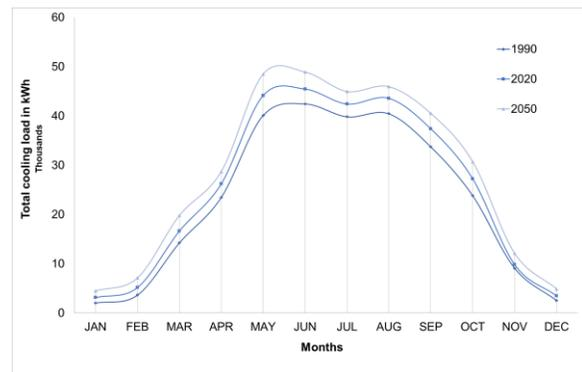
Figure 3: Cooling load in kWh for DA HQ building
