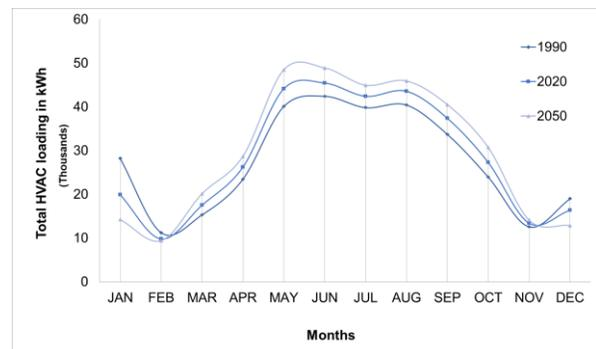
Figure 4: Total HVAC in kWh for DA building
